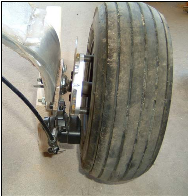
A Top View of the Brake Assembly
