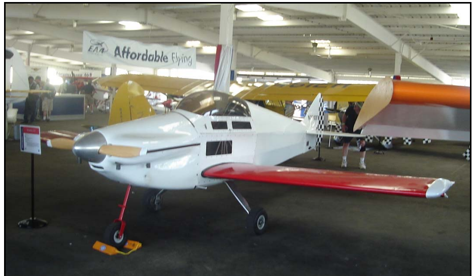
Tim Hoversten's Sonerai IILT in the Affordable Flying Center. This airplane started life as mid-wing taildragger
