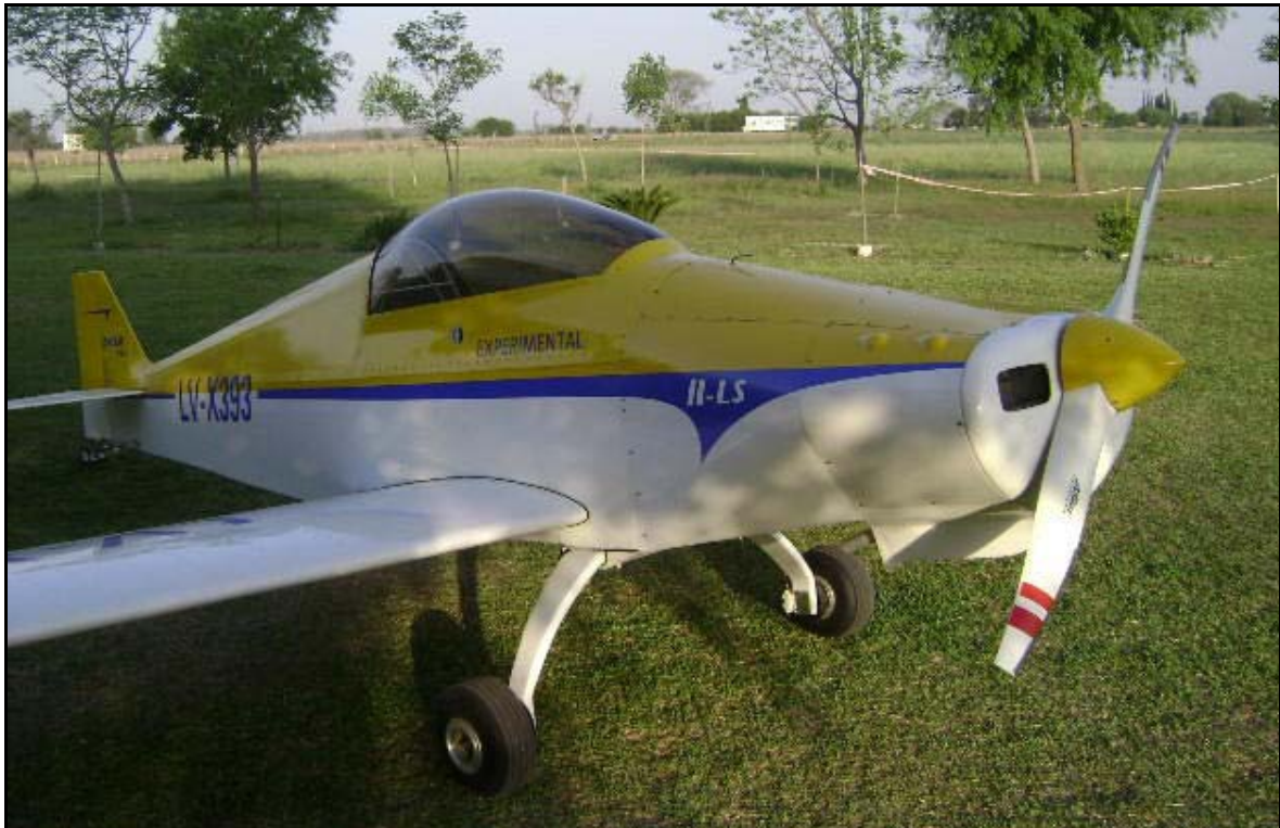
Hernan Marcos' Sonerai IILS As you can see by the registration number Hernan is from Argentina. The engine is a Continental A-75.
