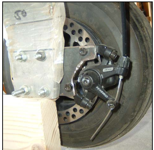
The Caliper Assembly
